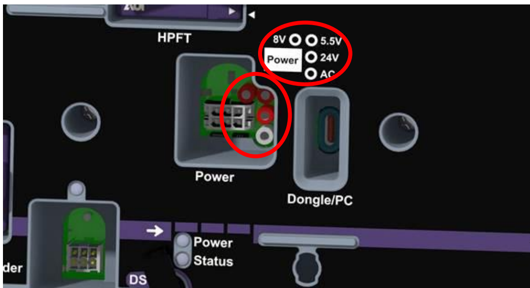
Figure 1- 6: AC/DC Test Point Locations
