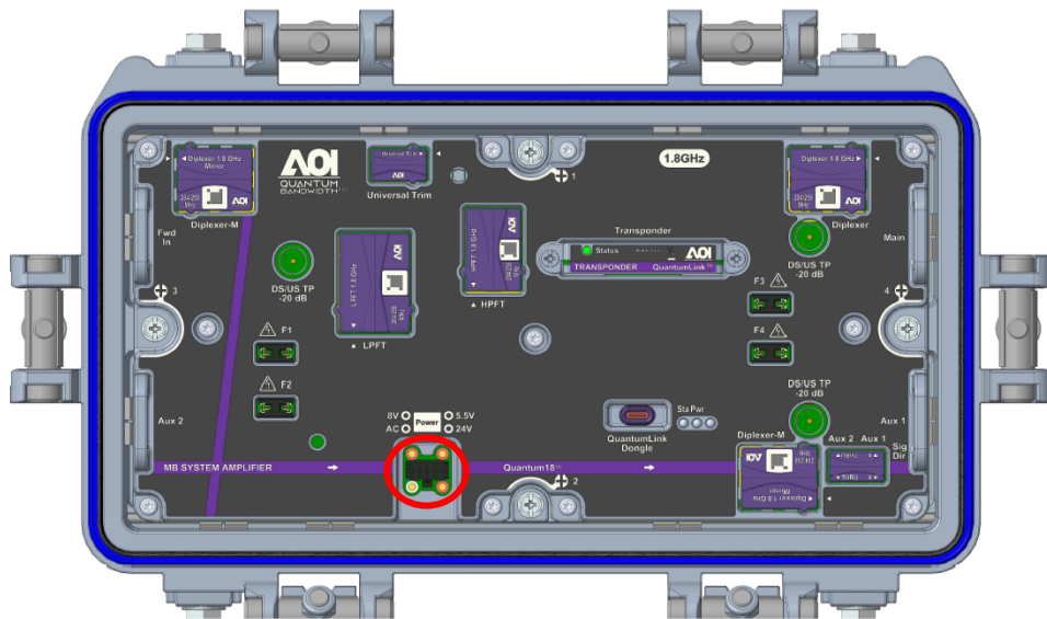
Figure 1- 4: AC/DC Test Point Locations
