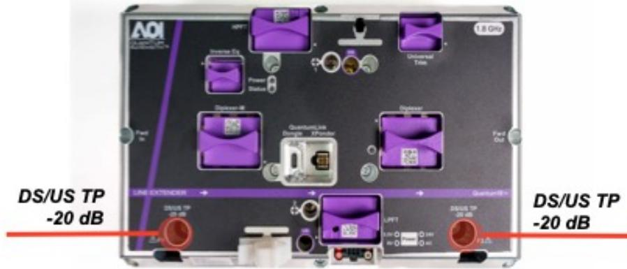
*Figure 1-1: RF Test Point Locations*
