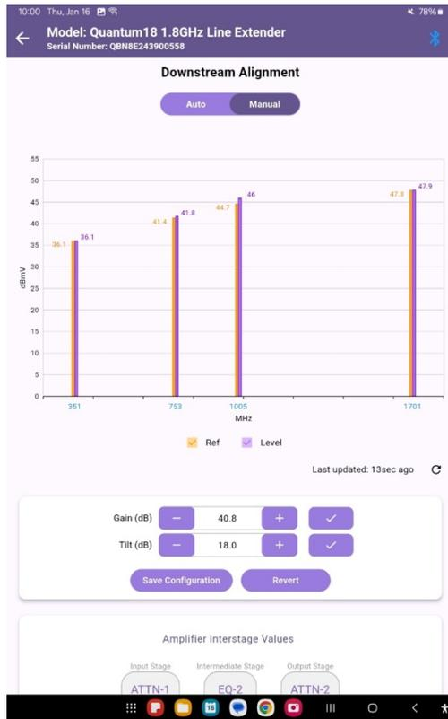
**Figure 3- 19: Downstream Alignment**
