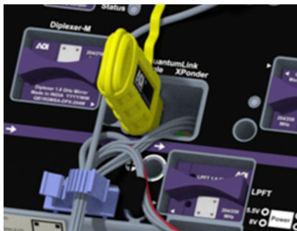
Figure 1-4: QuantumLink Local Wireless Interface
