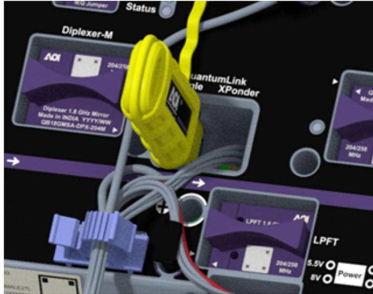
*Figure A- 3 QuantumLink Local Wireless Interface Installed in an LE*
