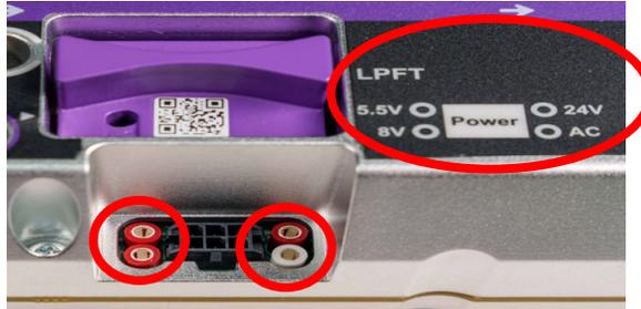
Figure 1-3. AC/DC Test Point Locations
