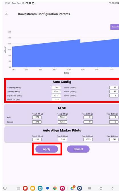
**Figure 3- 16: Auto Config Details and Apply**
