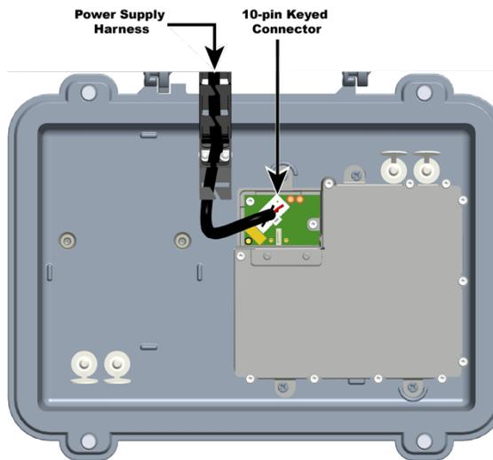
**NOTE:** The 10-pin keyed connector can be connected one way only. Be sure that the connector is installed securely to the power supply board.
