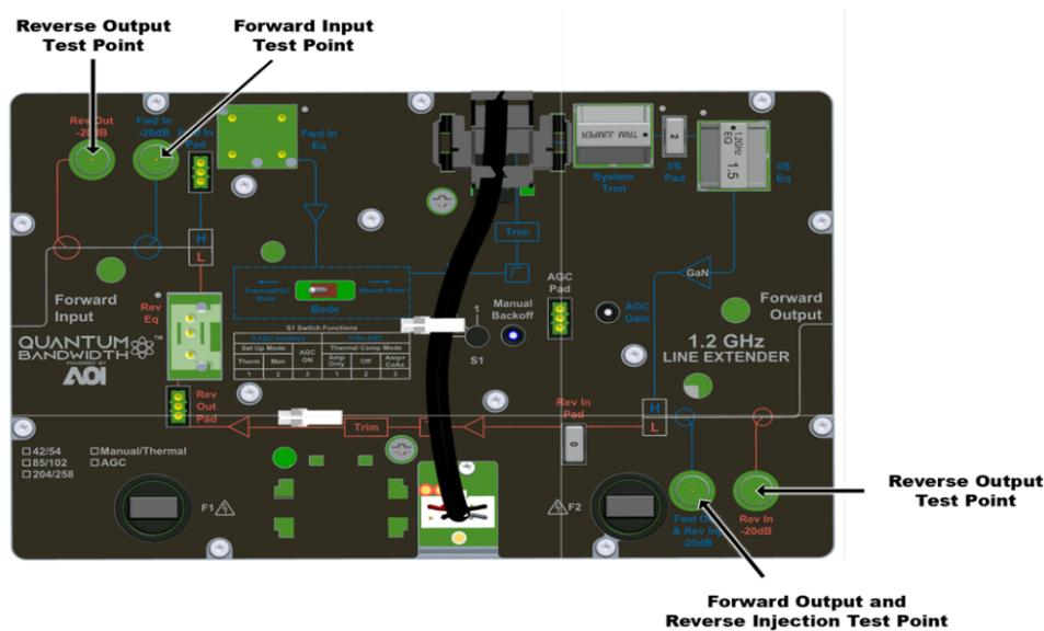
There are three voltage test points on the Quantum12 1.2GHz Line Extender power supply.
