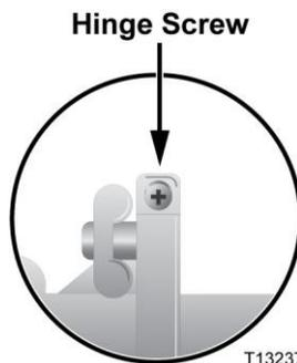
3. Using a screwdriver, remove the hinge screw from the housing hinge. The housing lid will now swivel completely open, allowing it to be removed from the housing base.
