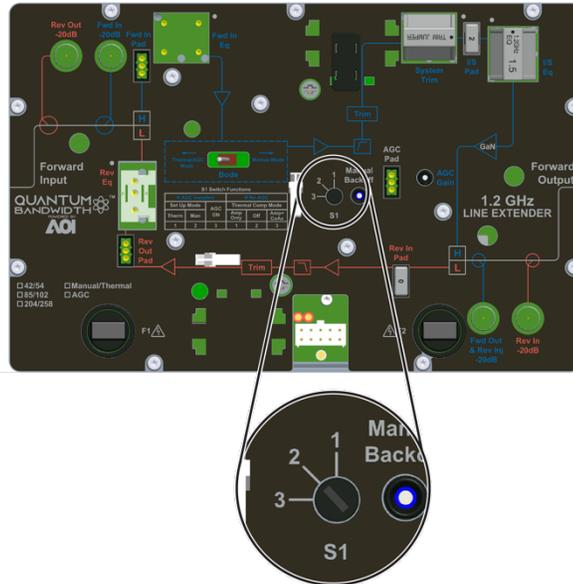
2. Insert the test probe into the -20 dB forward main output test point on the line extender.
