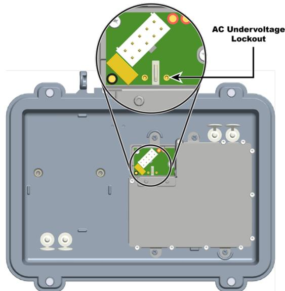
2. Set the AC undervoltage lockout selector for your powering application as illustrated in the following diagram.
