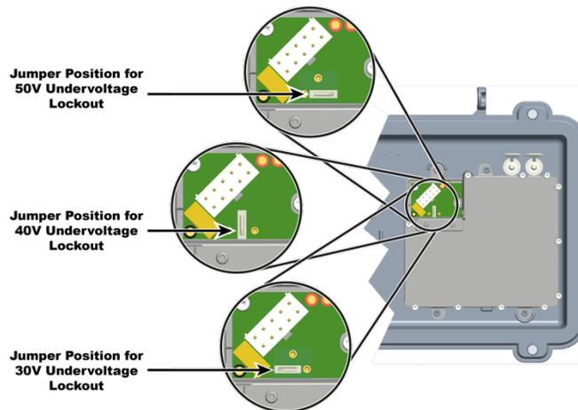
*NOTE: The AC undervoltage lockout selector positions are also noted on the power supply.*
