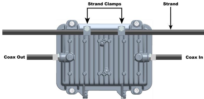
**NOTE:** Coax In may be switched with the Coax Out if you reverse the line extender module and feed the signal from right to left.
