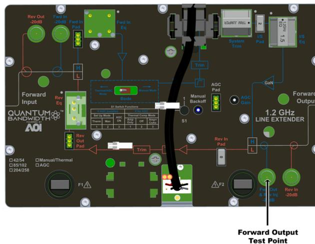
3. Measure and note the RF output level at the AGC pilot frequency.
